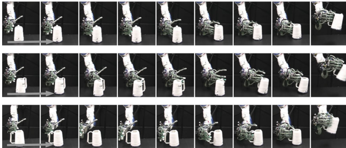
Fig. 5. Robot grasps objects using the trajectories learned during scaffolding. Each row corresponds to a different grasp execution.
